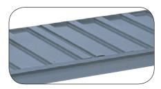
**Ribbed Decking -** Versatile 20-gauge ribbed decking. Ribs allow for space to grab packages easily and prevent pinched fingers. 13/4"w x 5/8"d rib.
