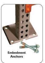
Bigfoot® Rack from Lyon gets its name from the oversized 8" x 6-1/2" x 3/8" all-welded footplate which anchors our 12-gauge steel, 55,000 psi upright posts. The 3" x 3" uprights are slotted to allow easy beam adjustment on 2" centers. 13-gauge bracing on 48" centers produces a structurally superior member with capacities up to 20,000 lbs.
