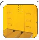
Heavy-duty ribbed, galvanized steel shelves deliver load capacity of 350 lbs. per shelf and are adjustable on 3" vertical centers
